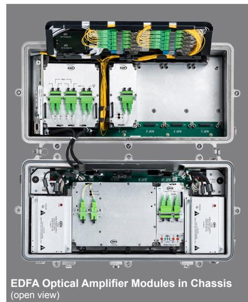
EDFA Optical Amplifier Modules in Chassis
