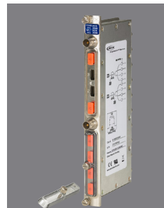
Passive Module with Make-Before-Break Attenuation (front view)
