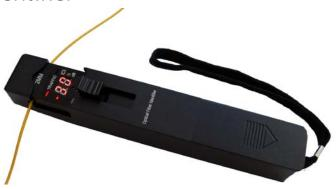
OFI-20A can detect optical signal presence, type and direction anywhere on fibers during optical network deployment, maintenance and troubleshooting. With non-destructive macro-bend detection technology, it introduces no damage to tested fiber or interference to the service on fiber. OFI-20A is able to identify wide-spectrum signals (such as signals in CATV system) and can be used in SONET/SDH & DWDM systems tests.
