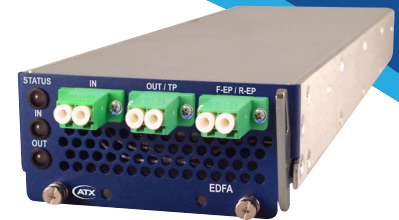
EDFA (front view)
