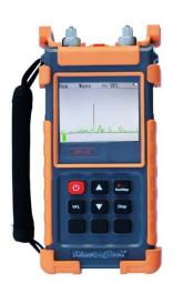
OFI-50 uses optical fiber sensing principle to confirm the target fiber; It can quickly identify deep buried, overhead and pipe fiber cable without any destroy, and provide a simple method for maintenance personnel. Users only need gently knock on cable, when knocking to the target cable, OFI-50 can clearly hear the knock from earphone, which can accurately identify the target cable.
