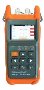
PPM-50 PON Power Meter can perform in-service testing of all PON signals (1310/1490/1550nm) on any spot of the network featuring pass-through design, burst mode and Pass/Warning/Fail assessment function, which can greatly help you evaluate PON signals transmission quality.
